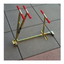
For extracting slabs it has a robust construction which enables the blades to be hammered between the joints.
